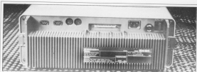
At the back of the machine there are five ports to play with including an audio/video connector and a serial port.
